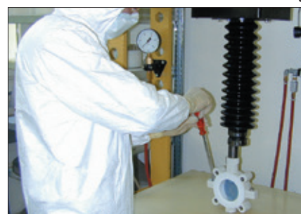
Valve assembly in clean room
