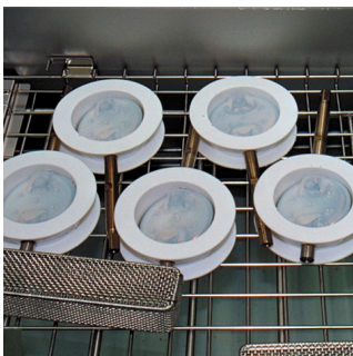
Cleansing the parts with ultrapure water
